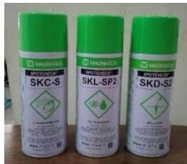
Gambar 5. Liquid Penetrant Testing
