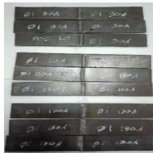
Gambar 3. Hasil Pengelasan Diameter Wire 1 Arus 90 A, 110 A, 130 A
