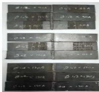
Gambar 4. Hasil Pengelasan Diameter Wire 1,2 Arus 90 A, 110 A, 130 A
