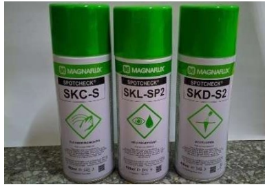
Gambar 5. Cleaner, Red Penetrant, Developer
