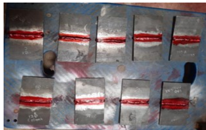
Gambar 6. Proses Pengujian NDT Liquid Penetran
