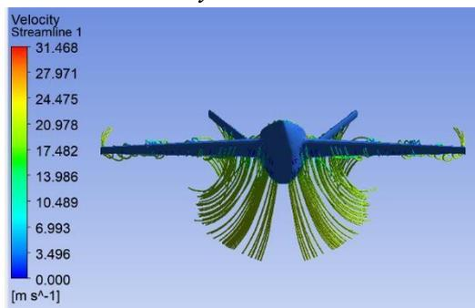
Gambar 29. Velocity Streamline 22 *m/s* melewati drone baru 15° tampak depan
