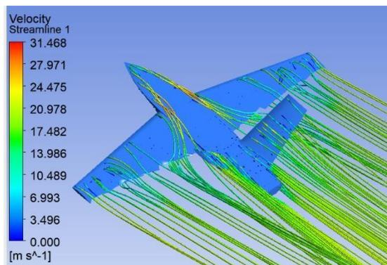
Gambar 32. Velocity Streamline 22  $m/s$  melewati drone baru 15° tampak Isometri
