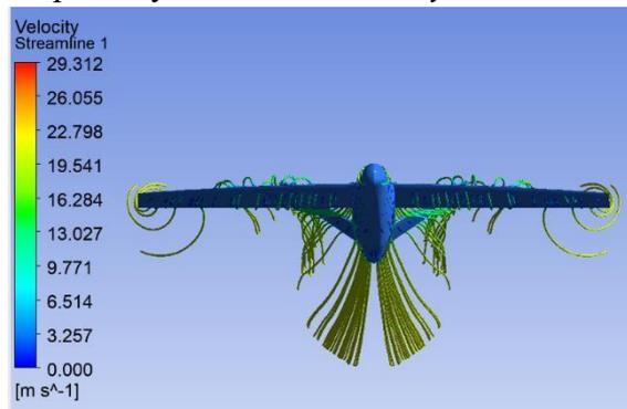
Gambar 23. Velocity Streamline 22 m/s melewati drone Airawata 15° tampak depan
