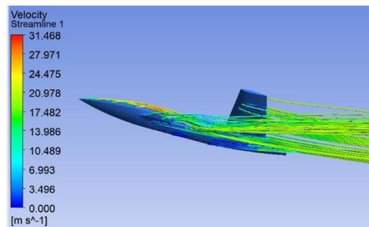
Gambar 30. Velocity Streamline 22 *m/s* melewati drone baru 15° tampak samping
