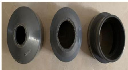
Gambar 3. Variasi Diameter Inlet Nozzel
