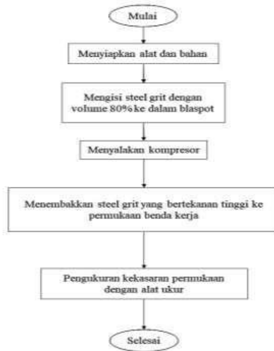
Gambar 4. Diagram alir proses sandblasting
