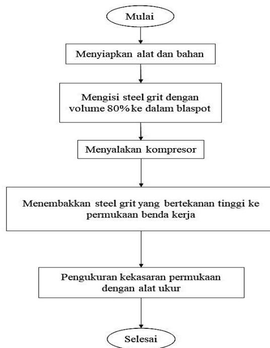
Gambar 2. Diagram alir proses sandblasting
