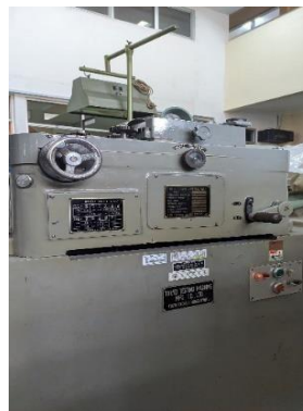
Gambar 9. Proses uji keausan Ogoshi
