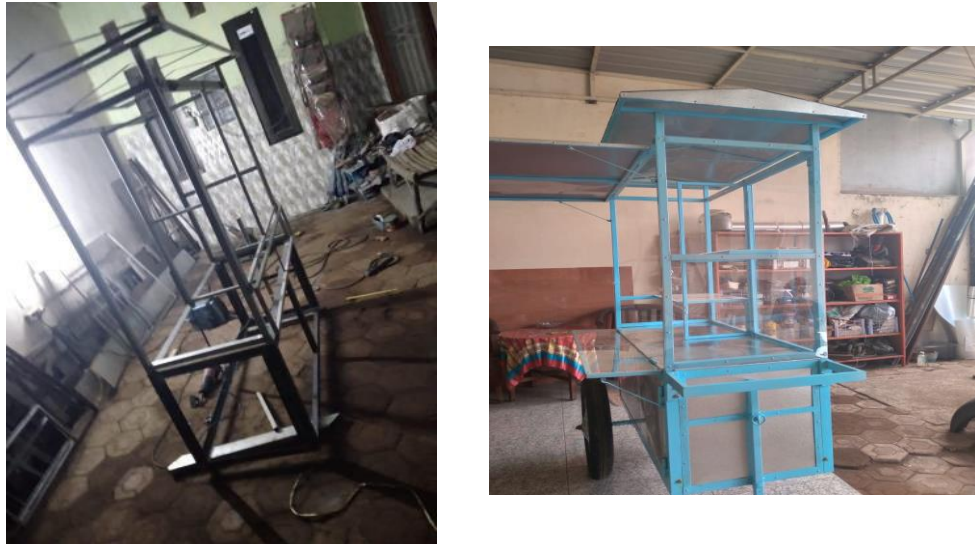
Picture 3. Knockdown cart manufacturing process
