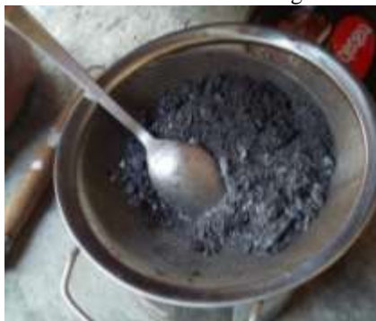
Fig 1d. coconut fiber ash is sieved on no. 100 sieve
